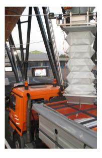
Round large silos with fully automated loading process and connection to the weighing system
