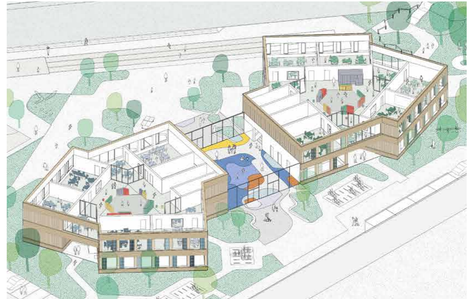
Draft of a cluster school with hybrid modular/elemental construction, created by Sauerbruch Hutton, Berlin.
